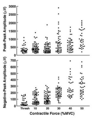
**FIGURE 5.** Needle- (upper graph) and surface-detected (lower graph) MUP amplitudes for two subjects at specific percentages of contractile force.
